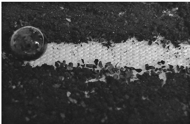
Fig. 6. Image showing the self-cleaning ability of a dusted modified cotton fabric surface.
